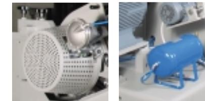
The SN is provided with a compressed air tank to keep the buffing pressure under control even in case of sudden falls of the air pressure. The reserve of compressed air allows the control of the emergency stop cycle of the machine even in case of air lack. The stop of the buffing roller is controlled by a disk brake.
