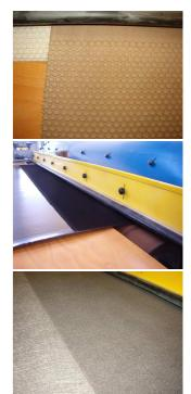
Other **special uses** of the belt buffing machine is on the **PU and PVC synthetic leather,** to get very uniform natural leather "nubuk" effect, with high production, regular quality and long life of abrasive papers.
