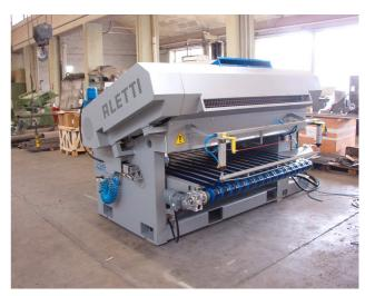
for **grain side and flesh side** buffing. The same machine can be used for an **aggressive buffing** (to get the surface of the product very rough to prepare the product for the application of cement and glue) and for a **very delicate and uniform buffing** (in case you need to improve the surface finish).
