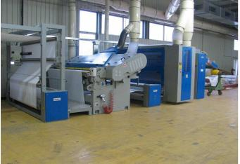
Besides the tannery and textile field, this machine is used for the deep engraving of car seats warp knit fabric upholstery, with the "pattern exclusive sueding" technology that enables to get permanent effects on the fabric without affecting original features.
