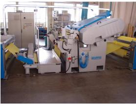
The precision and reliability of the end-less band buffing machine has allowed its use even for many kinds of **products in rolls** either for the **plain buffing** (nubuck, peach pile and velour) or for the exclusive "pattern buffing" (to reproduce on the surface of the product many types of designs only by an abrasive effect).
