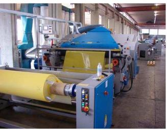
**feed in** (for most of textiles and for pattern sueding) and **feed out** (used for PU, PVC and sticky products (to get the buffing dust removed directly by the buffing machine, without need (in most cases) of any additional de-dusting.
