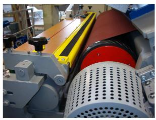
buffing roller. The temperature of the buffing roller keeps very near to the ambient temperature without the need for any cooling system. Consequently the performance of the machine is far better than the roller machine.
