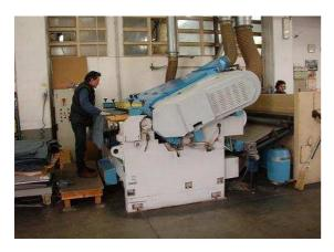
**6. Safer use and operation of the machine.** Thanks to the absence of longitudinal movement of the buffing roller, it is possible to fit a safety brake directly on the buffing roller shaft. The **disk brake can stop the machine in very short time**, in case of the operation of the safety device or in case of the interruption of power supply or a compressed air pressure drop. The **side replacement of the paper band protects the operator** from any contact with hazardous parts.
